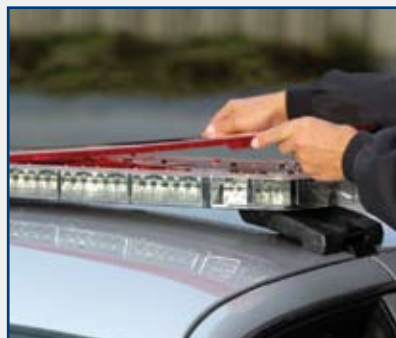
① Remove the top dome with only four screws.
