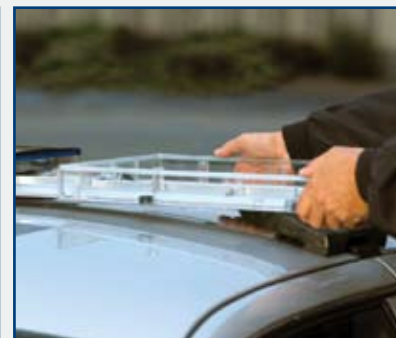
③ The base slides off for quick replacement.
