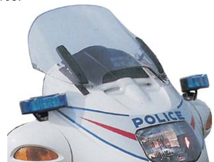
Sputnik LED lights installed on motorcycle fairing
