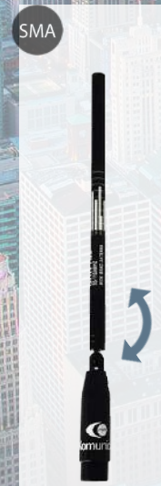
PWR-SRH-789 144-430 MHz RX-SCANNER 20-80.5cm Telescopic
